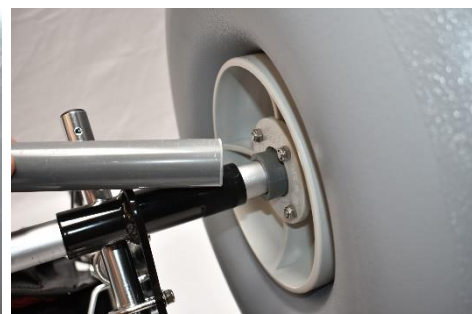
Check clearance and cut PVC to fill this area
