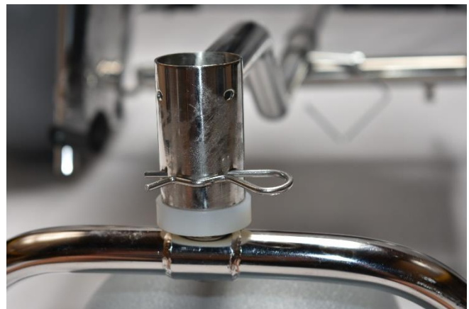
Reinstall hitch pin into bushing housing – ensure pin passes through both holes.
