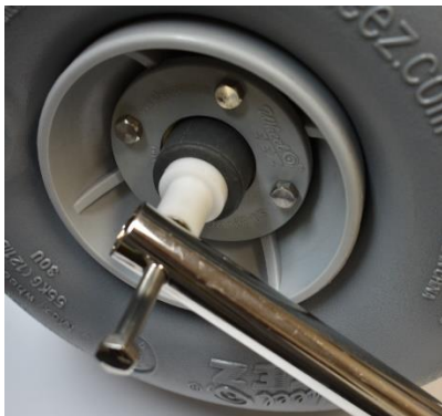
Position wheel between caster forks and install bolt
